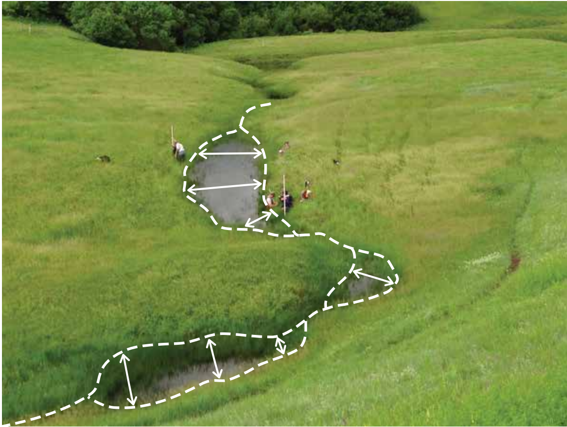
Figure I.9. Along a vegetated drainageway with discontinuous “necklace” pools, scour channels, or inundated flow paths, measure GGW at all sample locations. The greenline (dashed white line) follows the thalweg through the vegetated drainageways, and GGW is recorded as “0” in these sample locations. Through the pools, the greenline follows the water’s edge; GGW (white double arrows) is measured across the pool, perpendicular to streamflow or to the longitudinal axis of the pools if streamflow is not evident.
