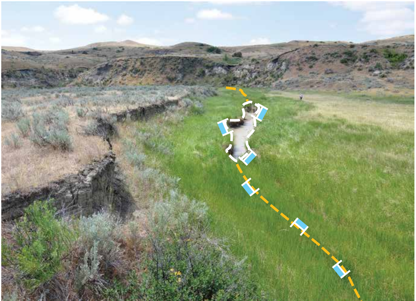
Figure 15. A vegetated drainageway with discontinuous pool or scour channel. The greenline follows the thalweg (orange-dashed line) through the vegetated drainageway but then splits to go on alternating sides of the scour channel or pool (white-dashed lines). Sampling locations alternate between left and right sides of thalweg or alternating sides of pools/scour channels.
