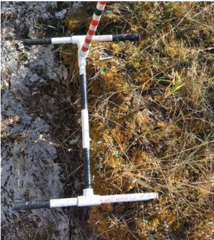
Figure D.9. Nonvascular plants such as moss and lichens (pictured here) are not considered part of the greenline. This moss would be considered a “bare patch” and the frame would be moved back away from the channel.
