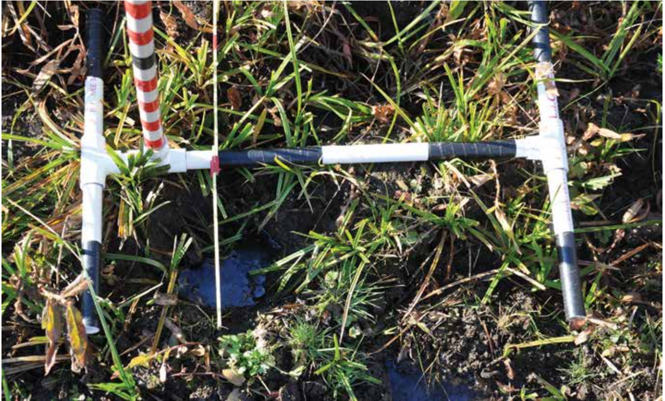
Figure 42. Using a ruler to measure streambank alteration. A folding carpenter's ruler is handy for simulating the path of the observation lines in the MIM frame to determine if these lines intersect an alteration. Note the standing water in the depressions created by recent hoofprints.
