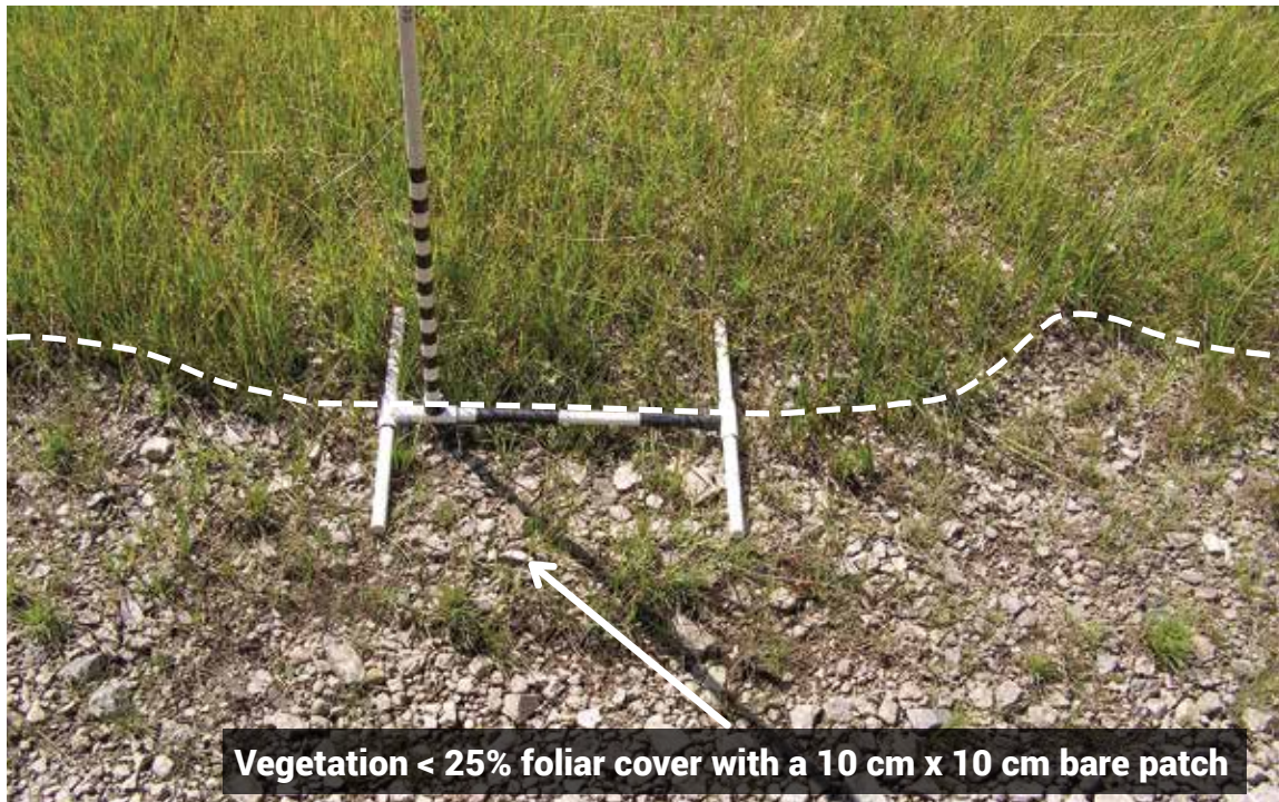
Figure D.5. Frequently the greenline is near the bankfull stage. The greenline cannot exhibit bare patches exceeding 10 cm x 10 cm. Bare patches are any combination of rocks smaller than 15 cm, litter, annual plants, dead plants that do not qualify as anchored wood, or nonvascular plants. The greenline here is located upslope of discontinuous vegetation patches that are closer to the waterline because that vegetation has < 25% foliar cover, with a bare patch of pebbles that exceeds 10 cm x 10 cm.
