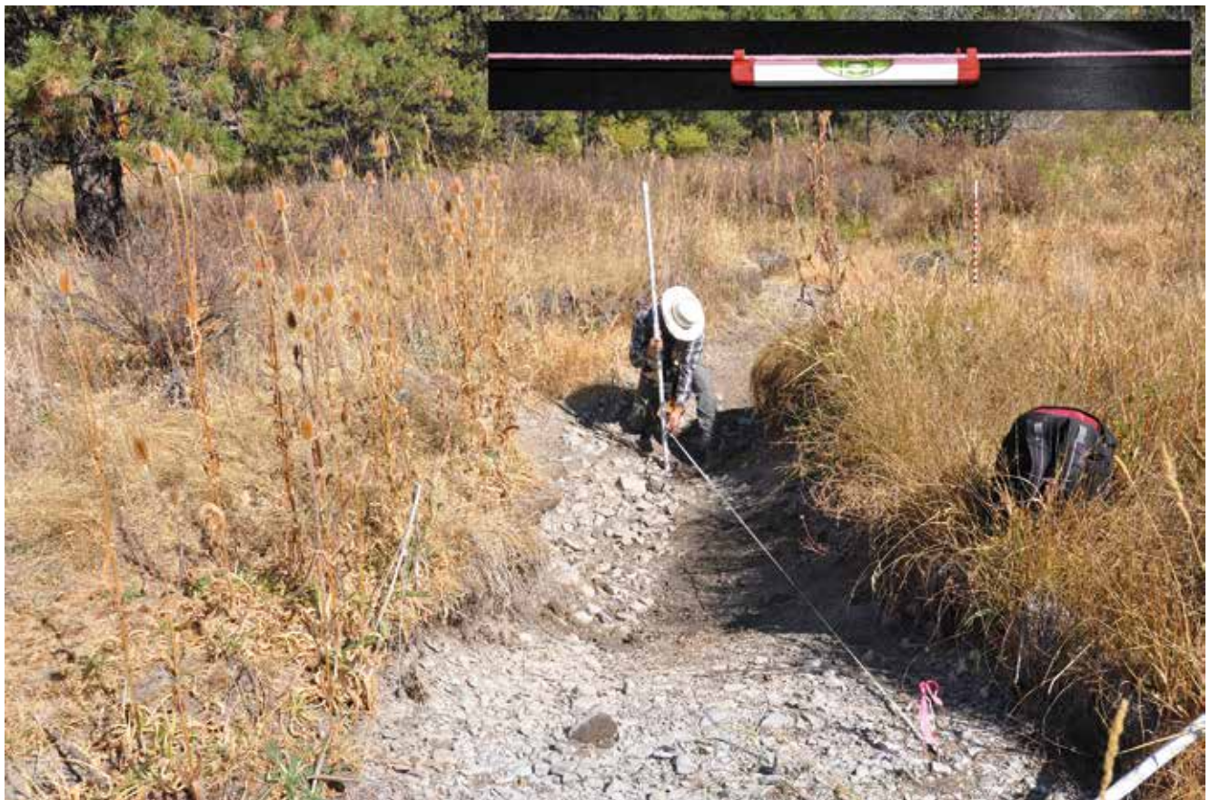
Figure 76. Measuring residual pool depth and pool frequency in a dry channel. Anchor or hold a tape, tag line, or mason line to the thalweg of the riffle crest (indicated by black arrow) and extend it to the pool bottom. Use a line level (example, upper right inset photo) to make sure the line is taut and horizontal. Measure the residual pool depth with a depth rod at the point the horizontal line intersects the rod (see person holding depth rod).
