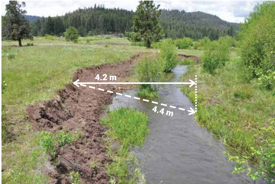
Figure 60. GGW is the horizontal distance between the greenlines on opposite sides of the stream channel. In this example, the GGW is 4.2 m (measured along solid horizontal line), whereas the slope distance (sloped dashed line) is 4.4 m. Vertical line is projected from the greenline to provide visual references of the greenline position in this channel cross section.
