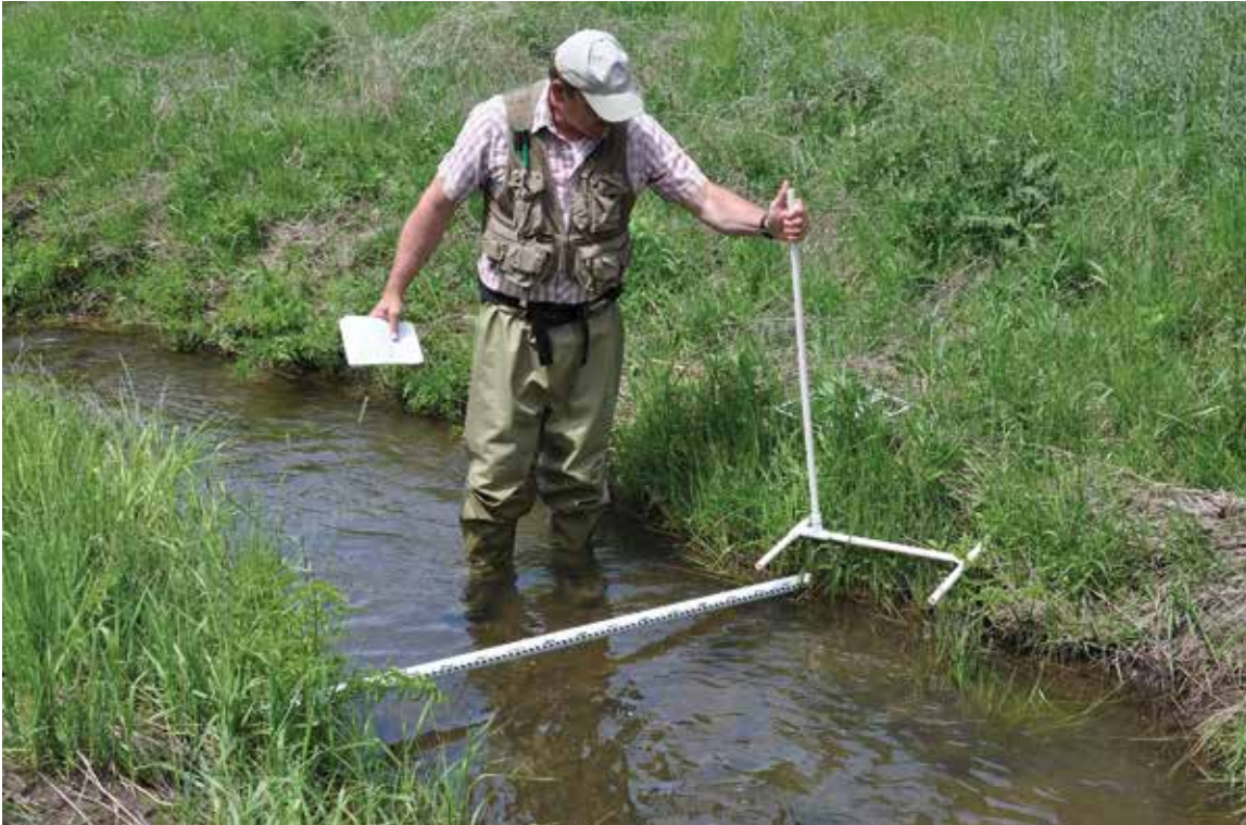
Figure I.3. In this image, the GGW is measured from the corner of the frame that is at the “start” or downstream end of the quadrat. This convention is especially important when the frame has been rotated so that it is not oriented parallel to streamflow.
