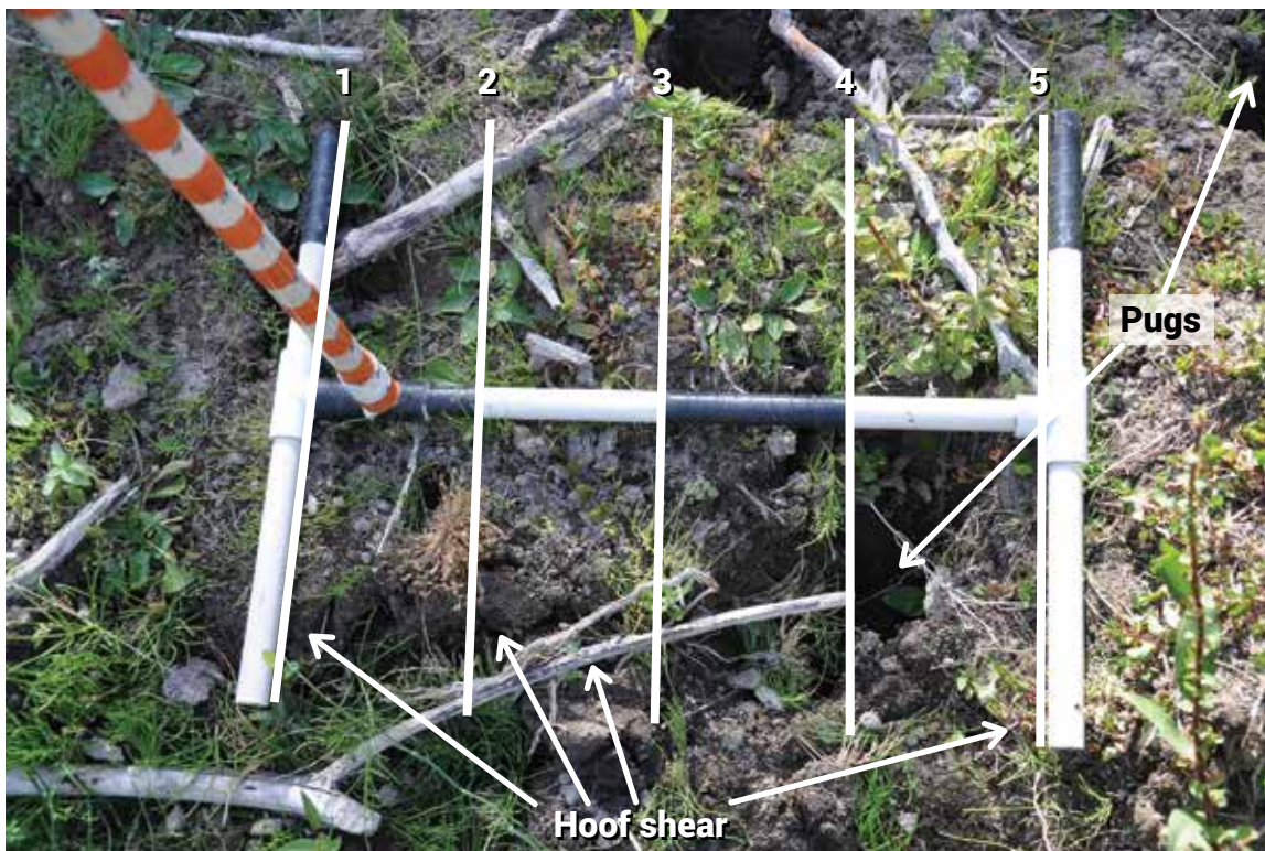
Figure E.3. Hoof shear has created a vertical face that intersects lines 1, 2, 3, and 5. Line 4 has a pug, or deep vertical hoof print. All 5 lines intercept an alteration, so 5 alterations are recorded.
