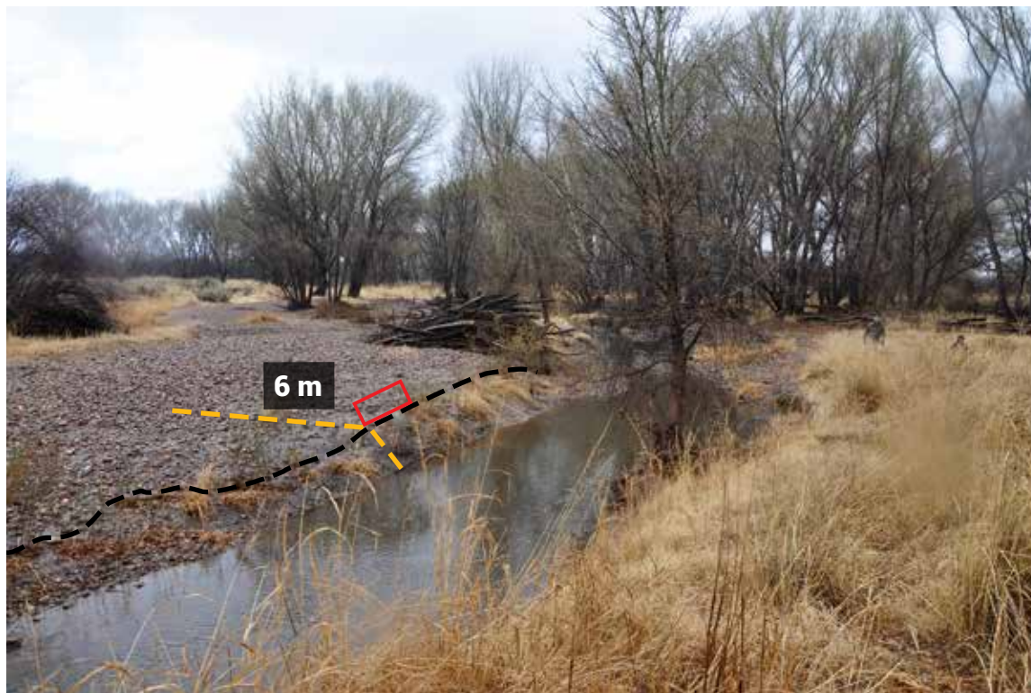
Figure I.6. When a greenline is not encountered within 6 m slope distance (orange dashed line) of the scour line (or edge of the active channel), the GGW is not measured—leave this indicator blank for this sampling point. The monitoring frame (red quadrat) is placed on the first bench (black dashed line) to measure other indicators (i.e., streambank alteration and streambank stability and cover).
