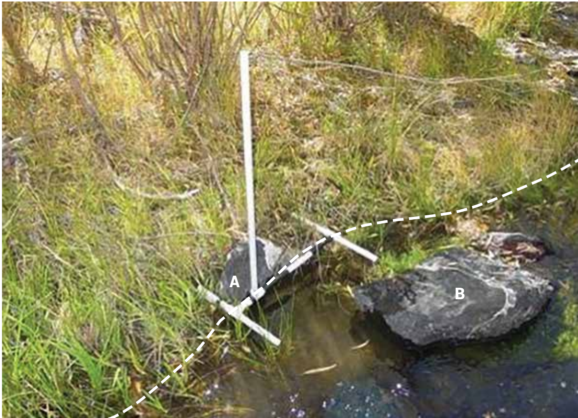
Figure D.10. Rock A is > 15 cm (intermediate axis), embedded, and is above the scour line, therefore, it is not considered a bare patch. Active erosion exists on the streambank side of rock B. The greenline is located as shown by the dashed white line.
