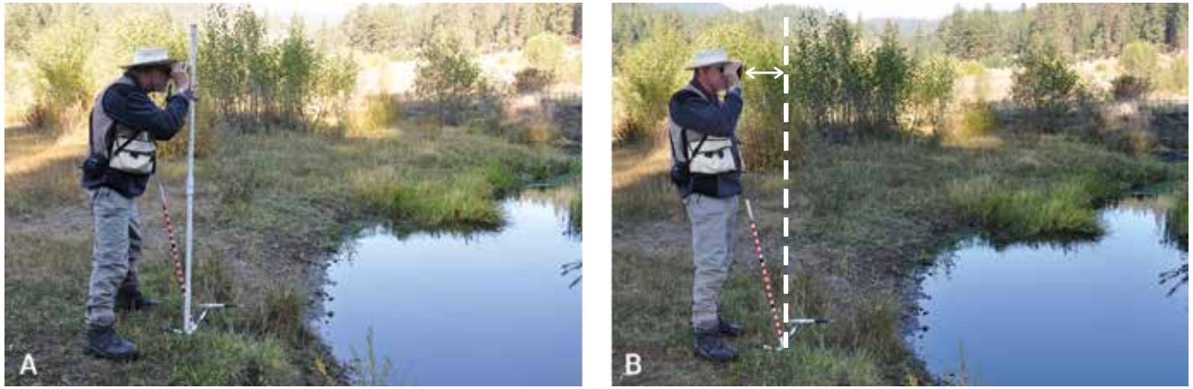
Figure 61. Examples demonstrating use of field equipment to obtain accurate GGW measurements.
