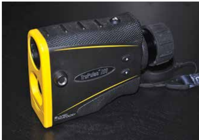
Figure 18. A precision laser rangefinder. The laser rangefinder is useful in laying out DMAs, measuring GGW and residual pool depth and frequency, and measuring the active channel width to collect substrate data.
