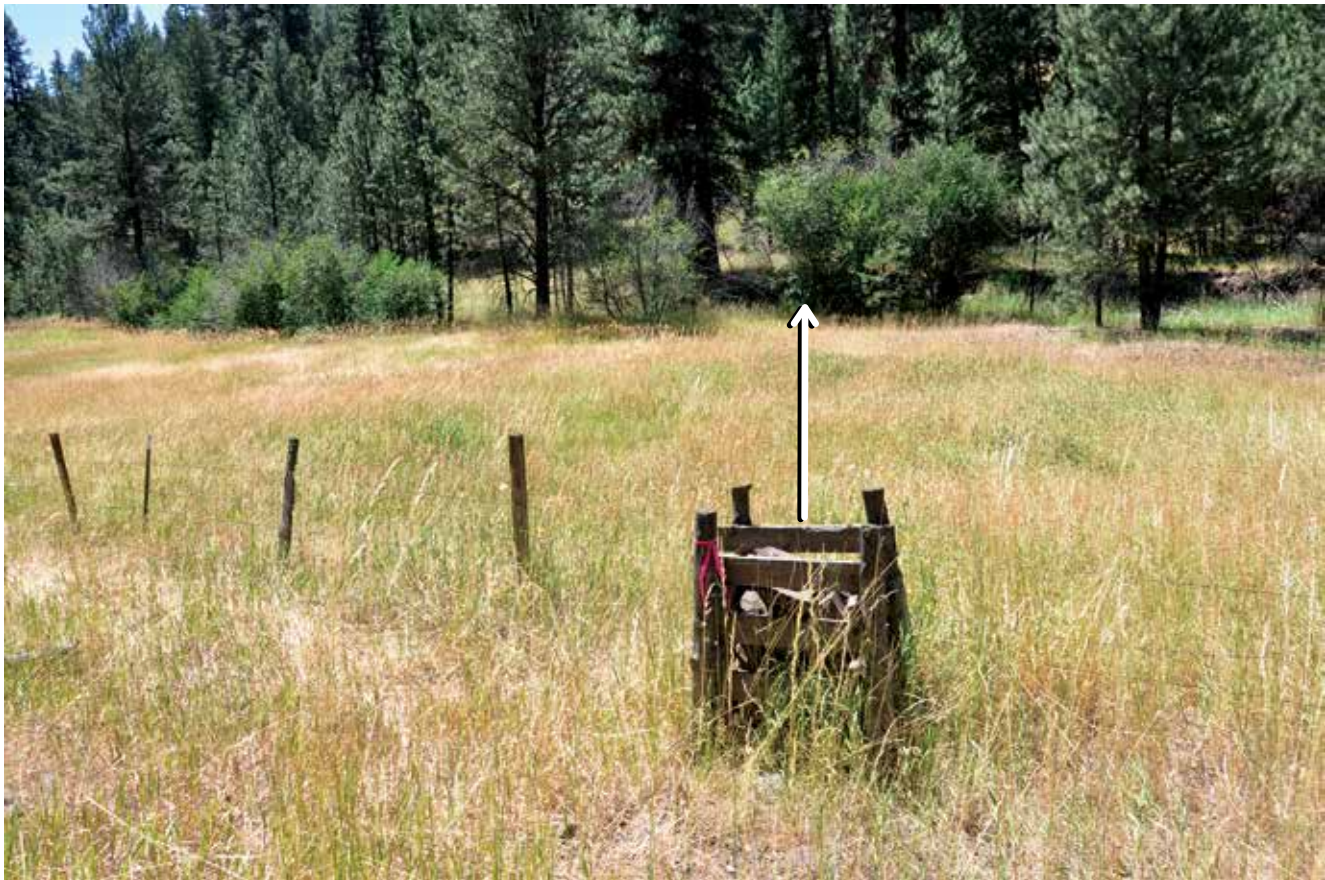
Figure 5. An easily identified, unique landmark or reference point is useful in relocating DMA markers. A single rock crib in a fence line within eyesight of the bottom of a DMA provides an unambiguous landmark to relocate a DMA marker. In this example, the azimuth (white arrow, 203 degrees) and distance (41 m) from the rock crib to the DMA marker have been recorded to facilitate relocation of DMA markers.
