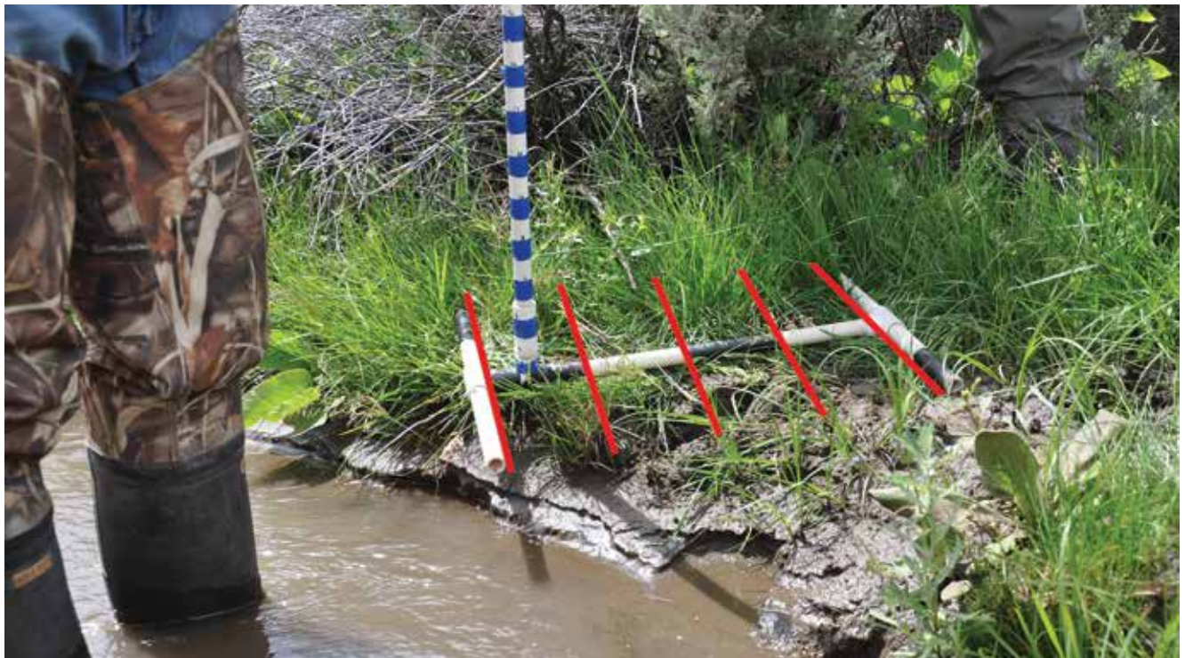
Figure 37. Streambank alteration is measured using a 42 cm x 50 cm monitoring frame. Five reference lines (shown in red) are projected across the width of the frame. Observation lines are 12.5 cm apart.
