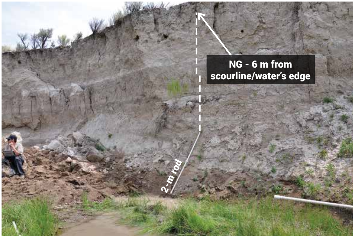
Figure 1.7. Although GGW is the horizontal distance between greenlines on each side of the stream, the distance measured to determine if no greenline (NG) occurs is based on ground, or slope, distance from the scour line or edge of the channel. Here, a 2-m rod is positioned with one end on the scour line and is aligned vertically up the face of a tall cut bank. The same 2-m increment is projected (white dashed line) to the 6 m distance from the scour line. It is impractical to locate the frame at the 6 m mark (vertical face). Because the 6-m mark falls on an inaccessible vertical face, the other indicators are estimated.
