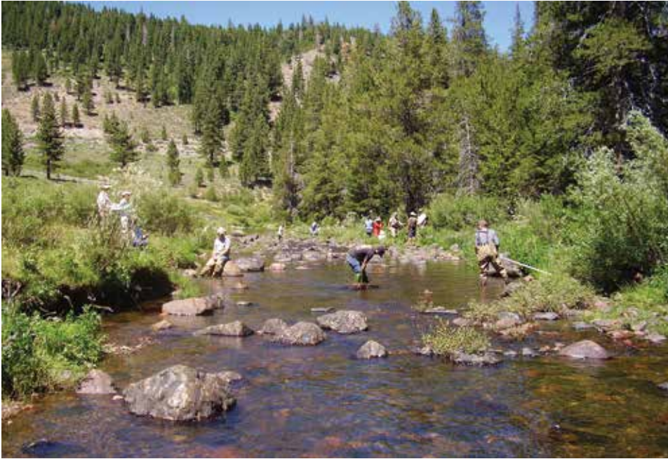
Figure 68. Excluding particles when measuring substrate. Boulders on the streambed that protrude above the scour line (which coincides with water surface in this image) and are not measured as part of the substrate.
