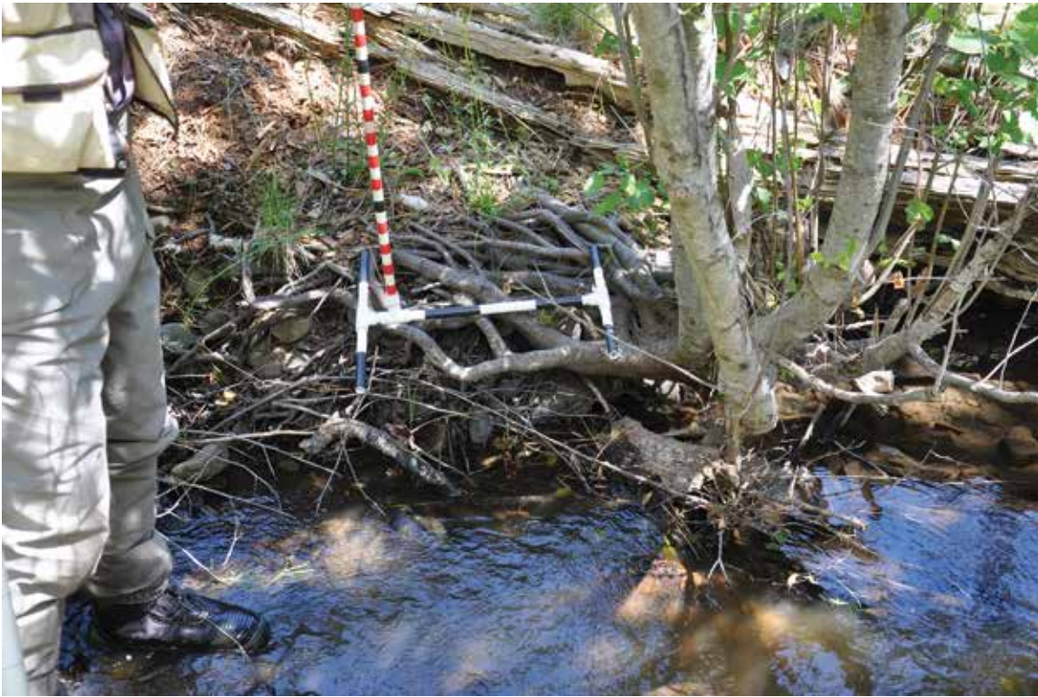
Figure D.17. Exposed live shrub or tree roots of overstory woody plants rooted in the ground above the scour line are part of the greenline (roots below the scour line are not part of the greenline). These are roots of overstory plants and the bare patch rule does not apply. Roots below the frame in this photo are not in contact with the streambank. The frame is placed where the roots are in direct contact with the bank.
