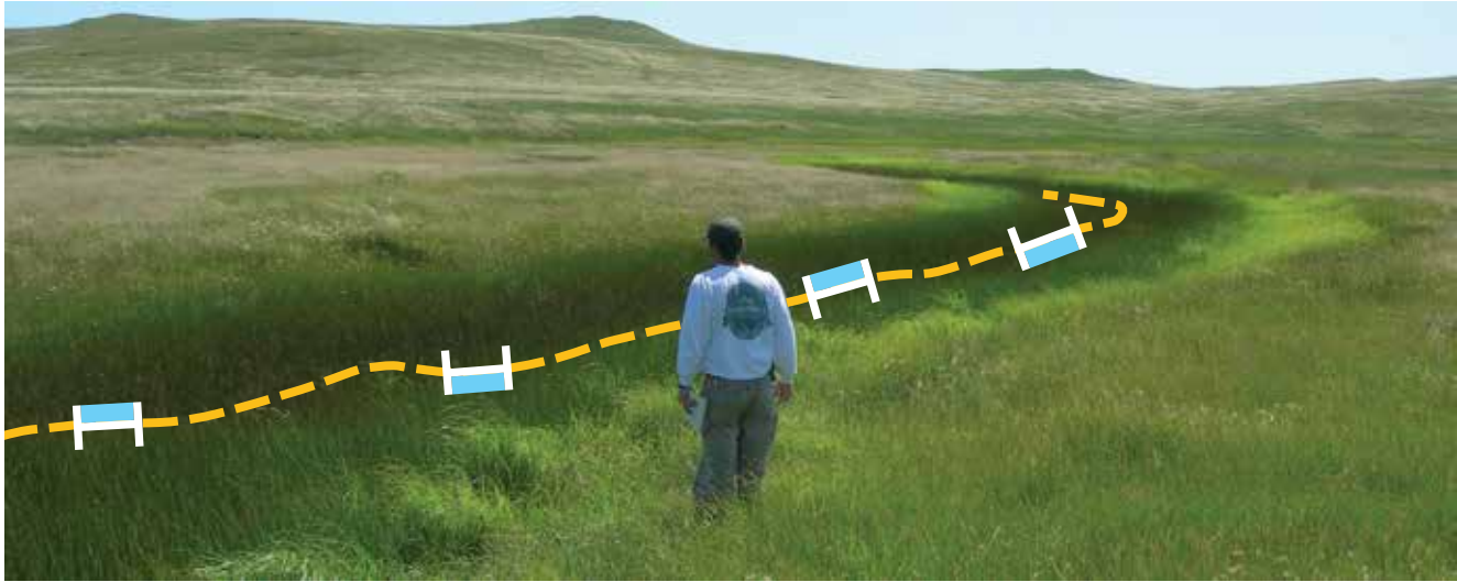
Figure 13. In vegetated drainageways, the greenline follows the thalweg (dashed line). Vegetation composition and cover, woody species height class, and stubble height are read in quadrats (see blue quadrats) on alternating left and right sides of the thalweg.
